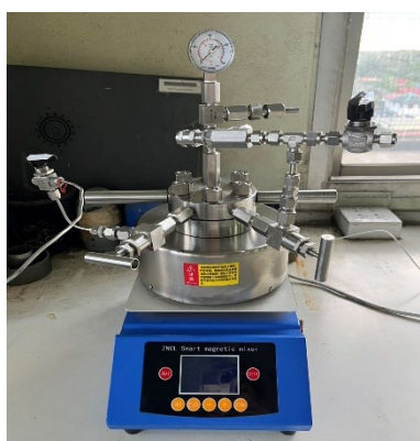
Figure 7 A photograph of a 100 mL stainless-steel autoclave reactor.
